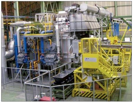
Figure 1. A new generation of automatic tending systems on rails are able to perform multiple functions, including charging, skimming, alloying, and furnace cleaning.
