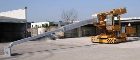
The long 'telescopic' arm allows for a comprehensive clean in even the deepest of furnaces
